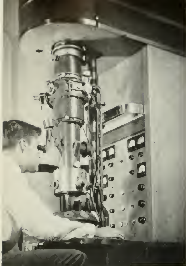
FIRST RCA ELECTRON MICROSCOPE TO BE BUILT (LEFT) WAS ACQUIRED BY THE AMERICAN CYANAMID COMPANY AND CONTINUES IN USE AS AN ESSENTIAL TOOL IN THE FIRM'S LABORATORY AT STAMFORD, CONN.
