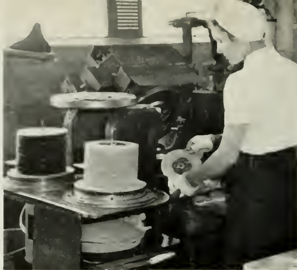
2 A 45-rpm record complete with labels is removed from one of the many powerful presses in the Indianapolis plant.
